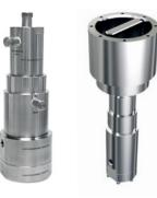
Designed to operate subsea at depths up to 3000m (10,000ft) these regulators can either use the external seawater pressure as a reference pressure or be completely sealed to operate at topside ambient pressure conditions, thus are completely unaffected by external pressure conditions. A version of the regulator is also available with a 'bucket handle' to allow subsea adjustment by ROVs.
